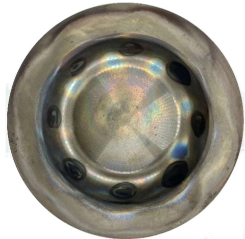
Figure 16: 422 piston, post engine test
